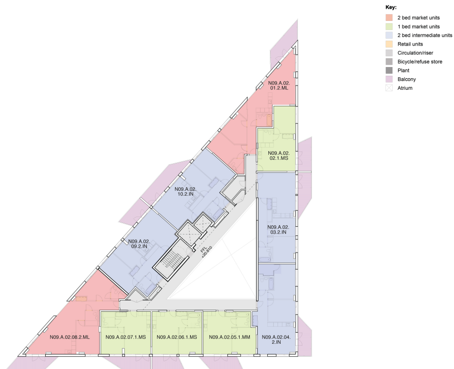
Fig. 14. Typical floor apartment layout and mix
